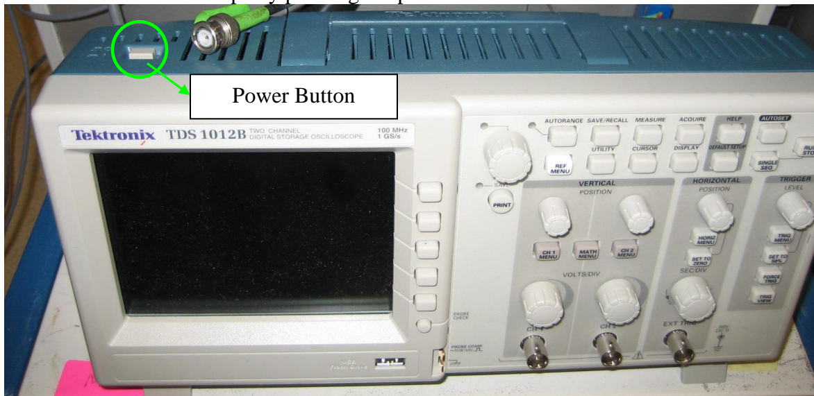
Figure 18. QMS oscilloscope emergency shutdown.
