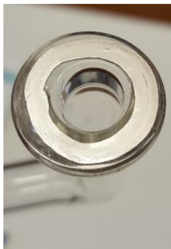
Figure 2.6: Photo of the flat glass flange connection with indium o-ring pressed flat after use (left) and the Delrin clamp (right). Photos by M. Nicewonger.
