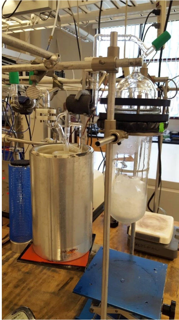
Figure 2.5: Photo of the extraction chamber (right) with an exploded ice core sample. The glass bead cold trap is immersed in the dry ice/ethanol bath (left). Photo by M. Nicewonger.
