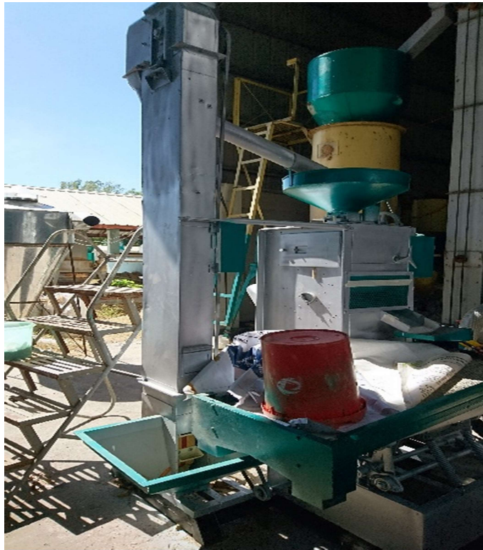
Figure 15: The prototype of the village-scale milling machine developed by PhilRice
