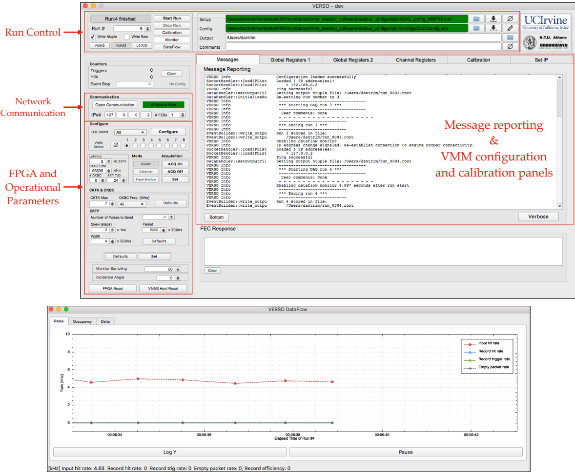
Figure 6.20: Top: Main VERSO user interface, with different logical blocks indicated. Bottom: VERSO dataflow monitor, showing the rate of VMM channel hits for all connected frontend boards and VMMs. Also displayed are the rate at which individual hits and events are recorded, where an ‘event’ is a collection of hits associated with the same trigger. The data being shown in this graph correspond to hits generated with the VMM channel test pulse injection with the output data recording disabled. The DAQ efficiency, defined in Equation 6.1, can be observed on this graph by dividing the blue line by the red line.
