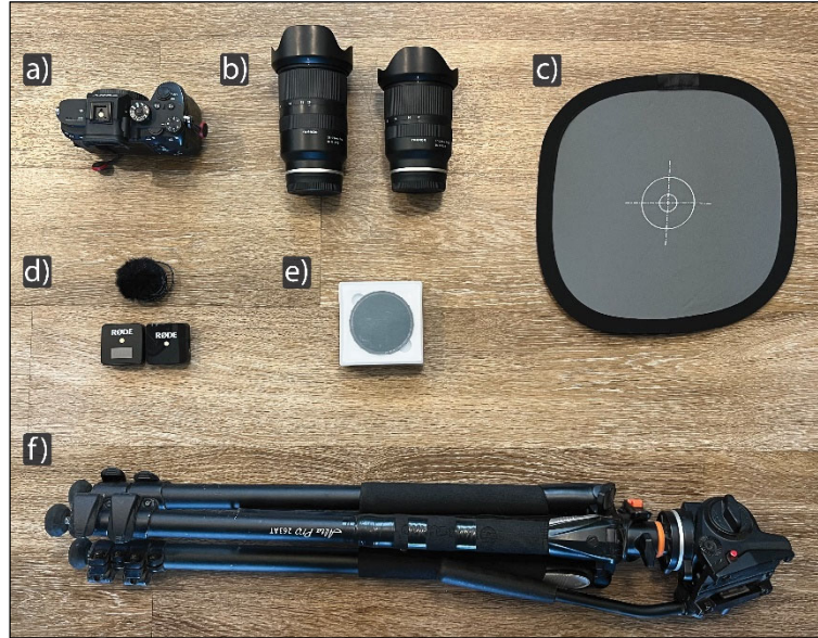
Figure 28: Camera equipment used for filming the field trip videos. a) Mirrorless DSLR camera body. b) Wide angle and standard zoom lenses. c) White balance card. d) Clip-on lavalier microphone and remote audio transmitter. e) Lens filters. f) Tripod with fluid head.
