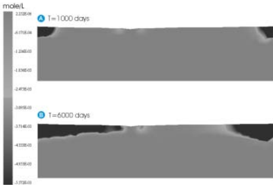
Figure 3-11. Computed results of pyrite concentrations for the first considered conjecture: upper boundary water is oxidizing. A) Computed results at 1,000 days. B) Computed results at 6,000 days. Comparison of both figures illustrates the advance of the pyrite dissolution front within the shallow fresh water system.
