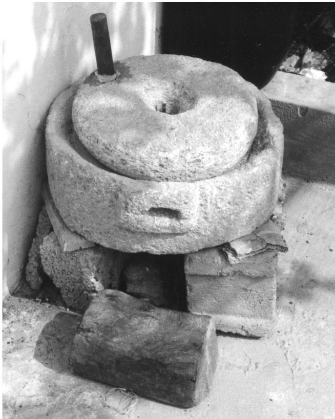
PLATE 6.20. The household handmill ( cheromilo ) used to grind grain for bread (in times of economic stress) and for everyday processing of hontro and pulses
