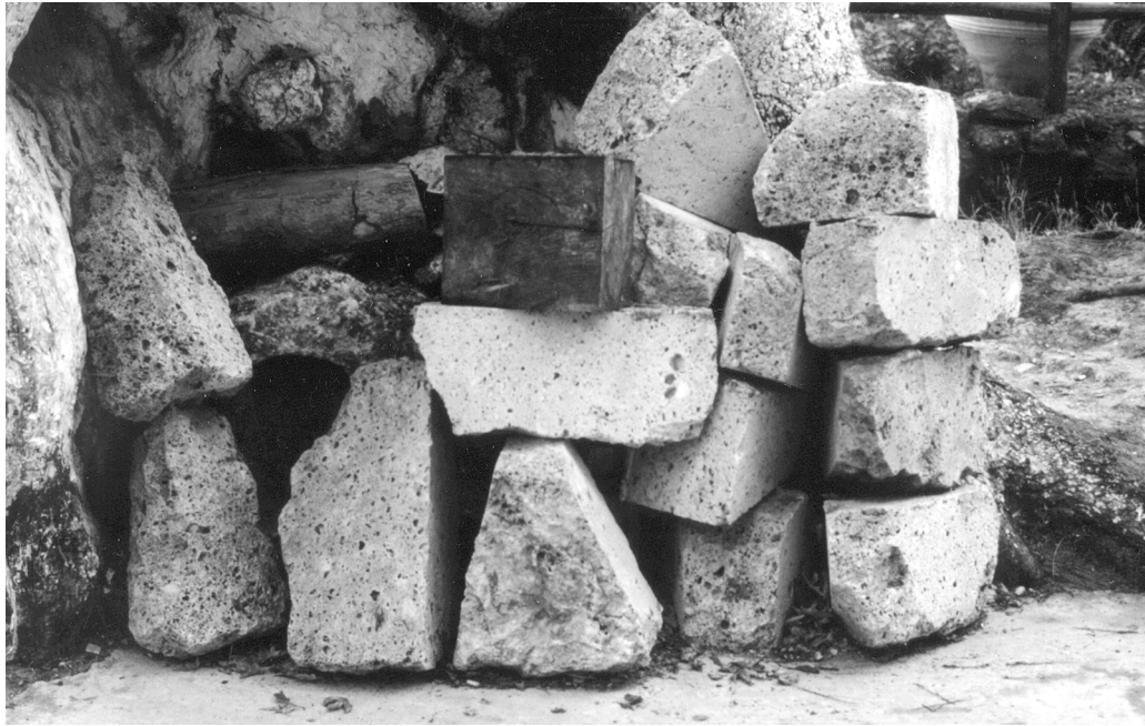
PLATE 6.17. Imported millstones ( mylopetres ) from Melos for the construction of a watermill. Shipped to Crete in pieces and bound with iron strips at the mill site.
