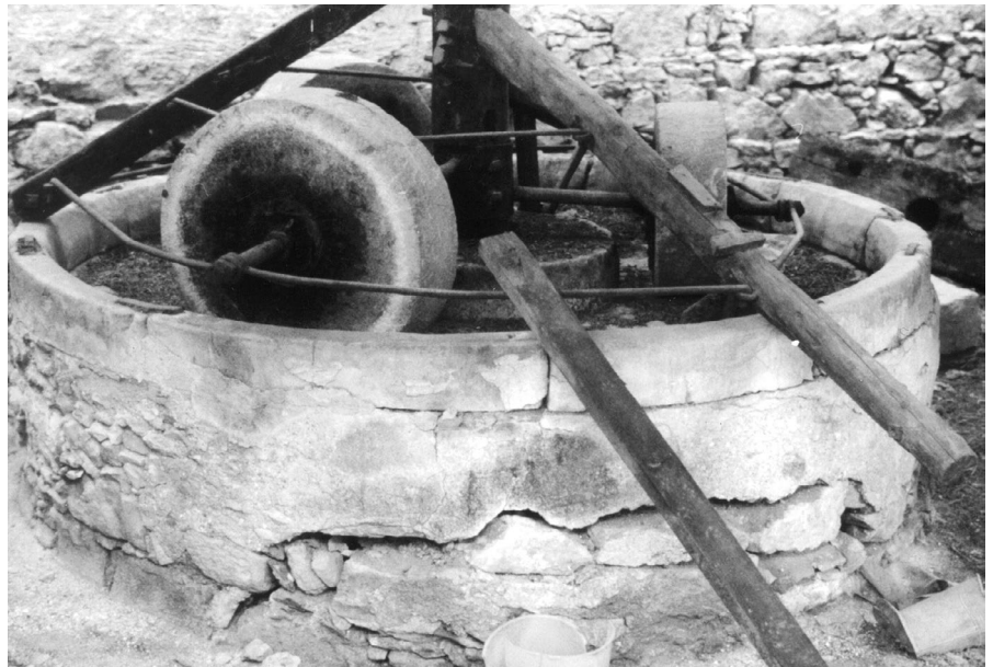
PLATE 6.33. The animal-driven aloni or stone crushing bed with three locally made mill stones in the Sivas oil mill
