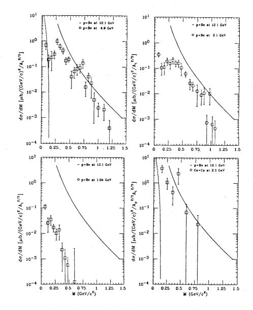
measurement of a cross section for pairs with a 1.0 Ca/A beam, where a clear pair signal has been measured.
