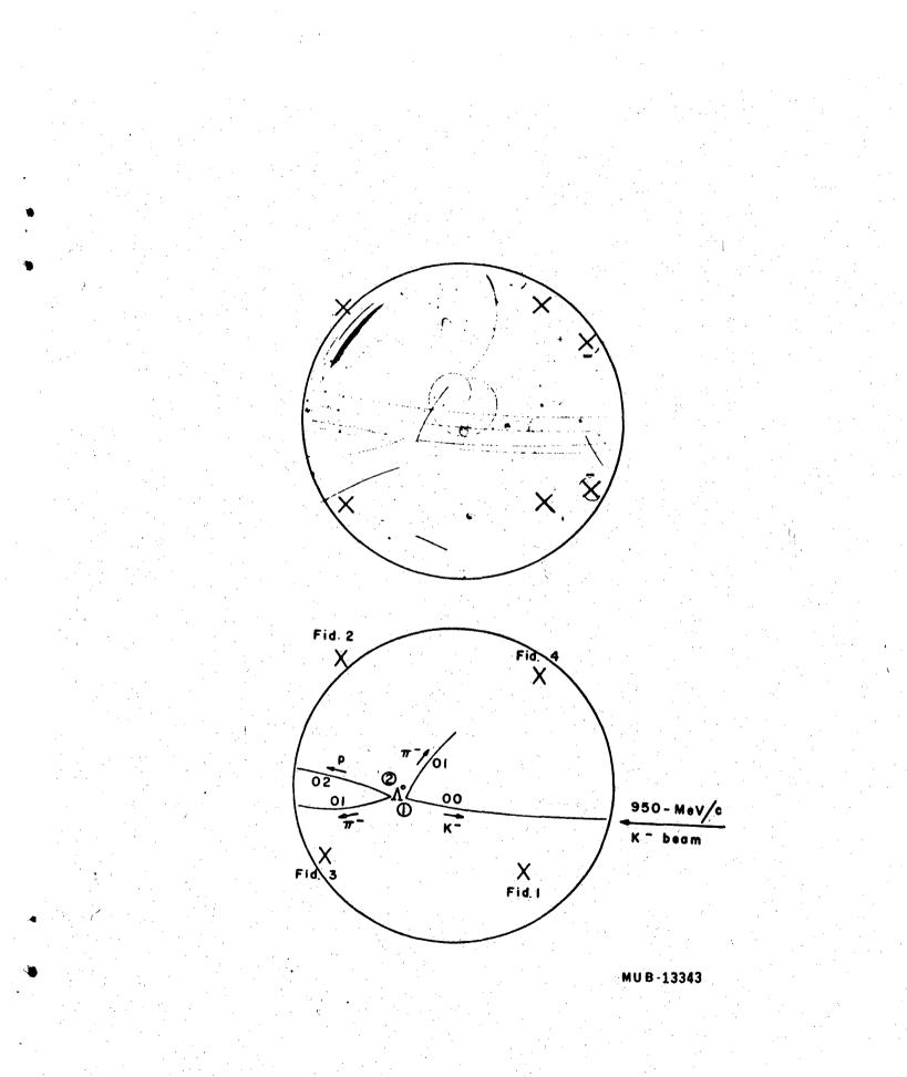
Fig. 2. Typical bubble chamber view showing fiducials and vertices.
