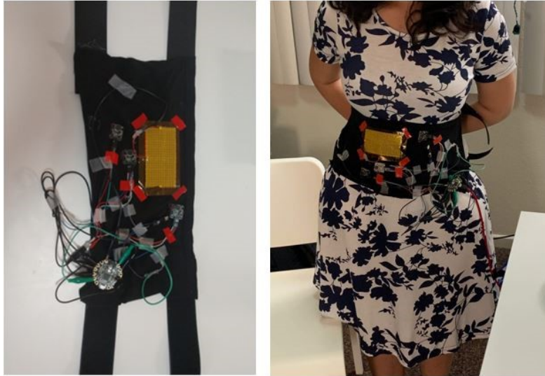
Figure 27: The belt with the vibration motors and Flora
