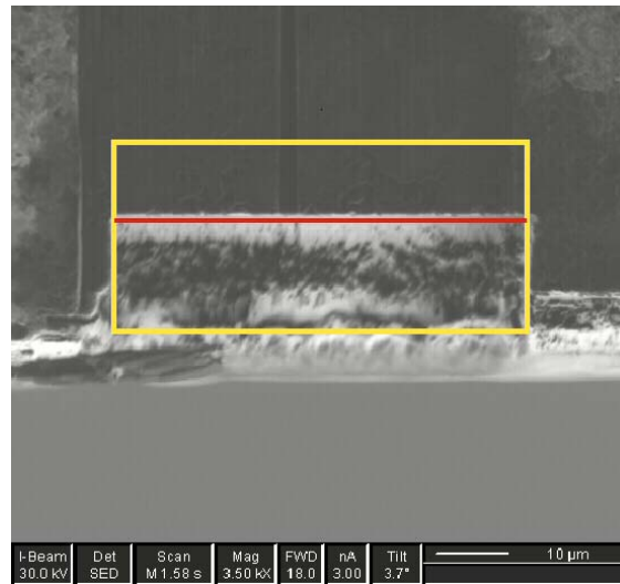
Figure 4. View from the ion beam direction of sample surface A during milling. The milling boundary is defined by the yellow rectangle and the most recent surface exposed is marked by the red segment
