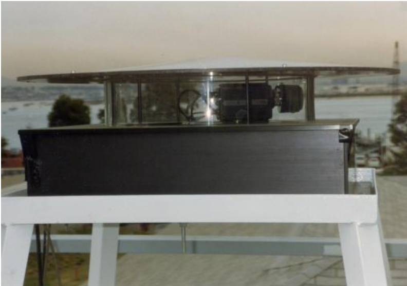
Fig. 2-1. Horizon Scanning Imager developed in late 1980's for determining Visibility
