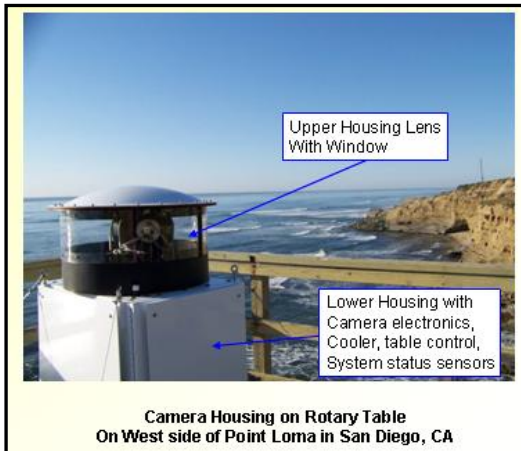
Fig. 6-4. MSI System on Pier
