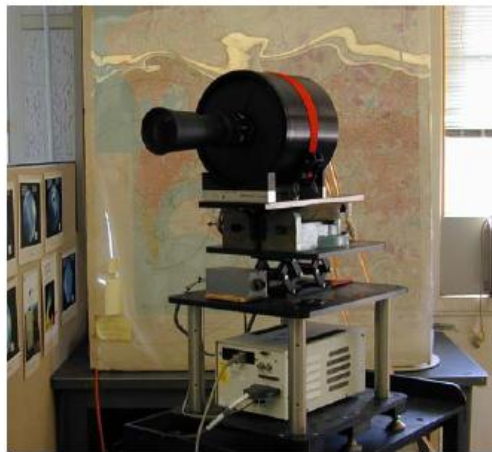
Fig. 4-1. MSI sensor head, Zuniga Shoals Project, with zoom lens and 16-bit CCD camera
