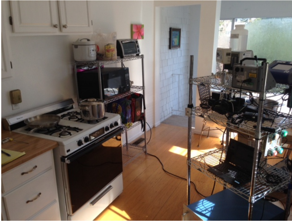
Figure 15. Positioning of kitchen instrument cart and gas range in H3. Note the pot and pan in position to be used for a simulation cooktop experiment.
