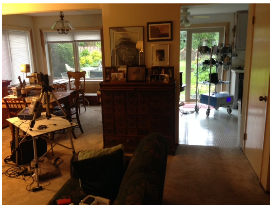
Figure 3. Air quality measurement instrumentation at central location (table) and kitchen of H9. Passage between kitchen and dining room (left, background) is of similar size to kitchen entry shown.
