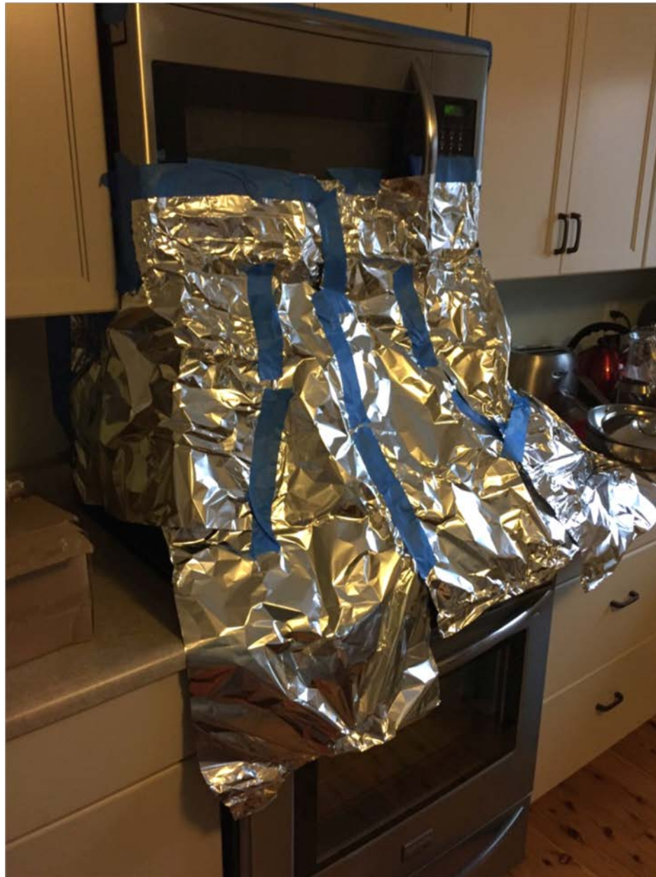
Figure 9. Range hood in H2 set up for first part of capture efficiency test.
