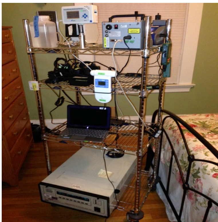
Figure 2. Air quality instrument cart in bedroom of H1.
