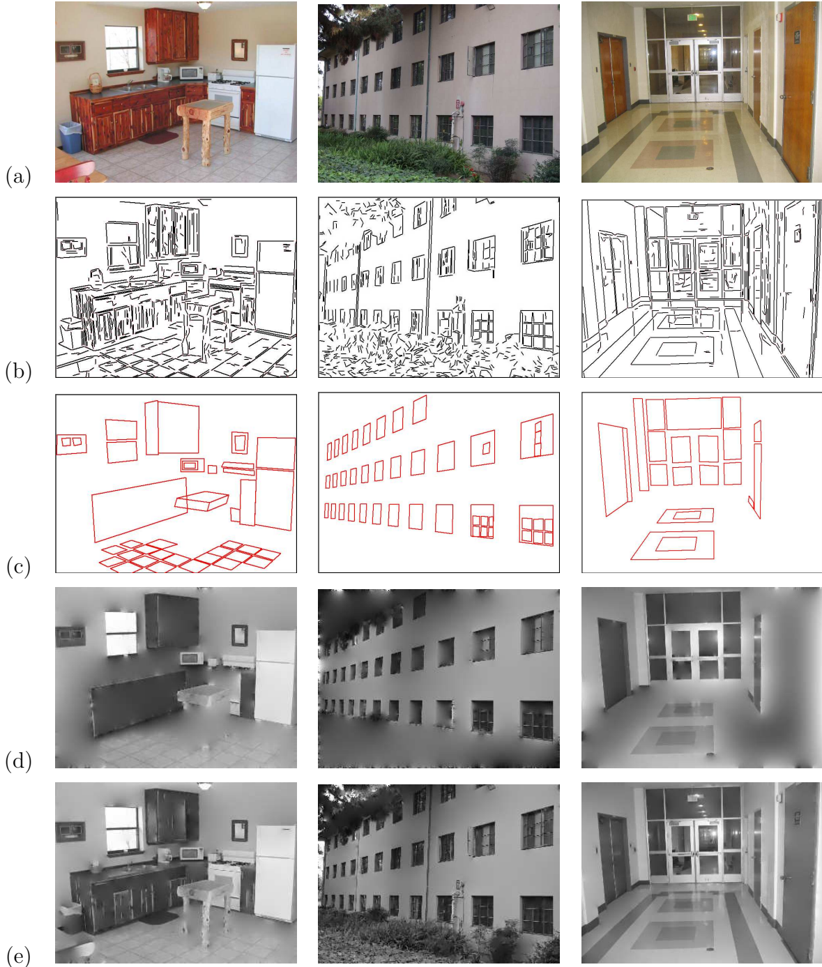
Fig. 11. Some experimental results. (a) Input image. (b) Edge map. (c) Computed rectangle configurations. (d) Reconstructed image from the primal sketch model using the rectangle configurations only. (e) Reconstructed images after adding some background sketches to the configurations.
