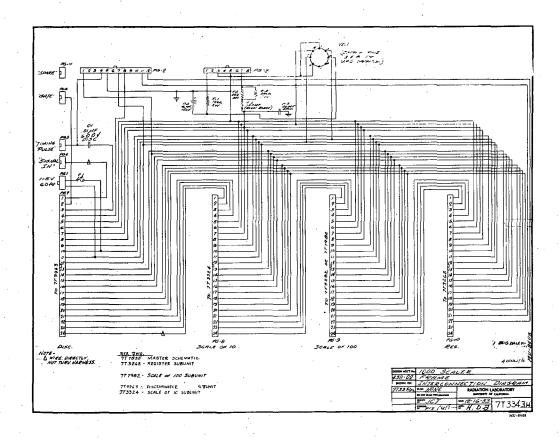
Fig. 14. Interconnection diagram for 1000 scaler.
