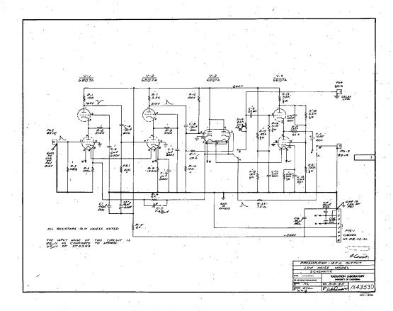
Fig. 11. Low-noise model preamplifier (125 $\Omega$  output).
