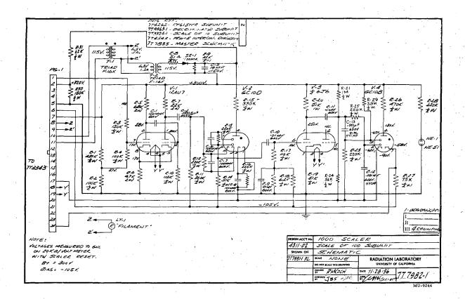
Fig. 17. Scale-of-100 subunit of 1000 scaler.
