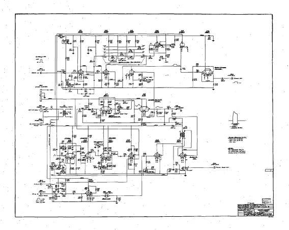
Fig. 13. Pulse shaper and timing-pulse generator, Model II.
