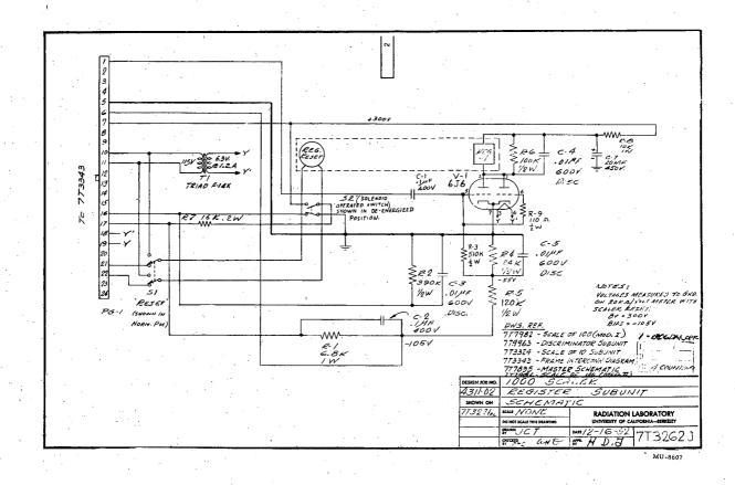
Fig. 18. Register subunit of 1000 scaler.
