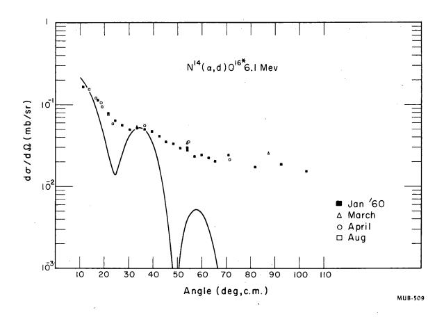
Fig. 8. Angular distribution of deuterons from formation of the 6.1-MeV level(s) of 0<sup>16</sup>. The solid line was calculated from the Glendenning equation by using  $j_n=1/2$ ,  $j_p=5/2$ ,  $R_0=6.20$  fermis.
