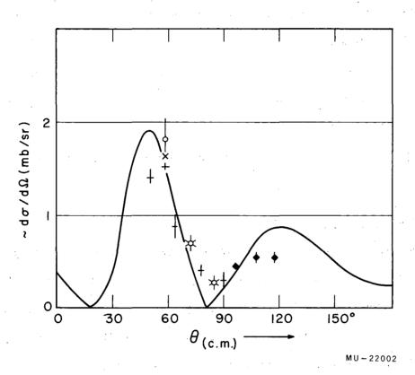
Fig. 10. Reproduction of the deuteron angular distribution from the Li  $(\alpha,d)$ Be $^{8}$  g.s. transition with ll.5-Mev helium ions. The solid line was calculated by using Butler theory for a knockout reaction; L=0, R<sub>0</sub>= 8.5 fermis. (After Starodubtsev and Makaryunas, Ref. 5.)
