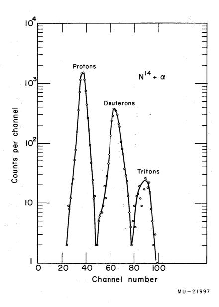
Fig. 2. Pulse multiplier spectrum from bombardment of  $N^{14}$  with 46.5-MeV helium ions.
