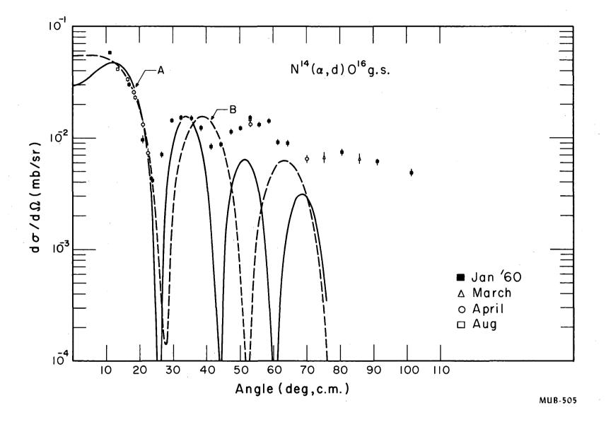
Fig. 12. Angular distribution of deuterons from formation of the ground state of  $0^{16}$ . Curve A was calculated from the Butler equation by using stripping parameters and L=2,  $R_0$ = 7.1 fermis; curve B by using knockout parameters and L= 0,  $R_0$ = 5.6 fermis.
