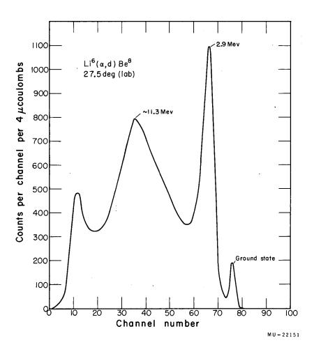
Fig. 3. Deuteron energy spectrum from the reaction Li  $^6(\alpha,d)$ Be  $^8$ . Q values for the various peaks are shown.
