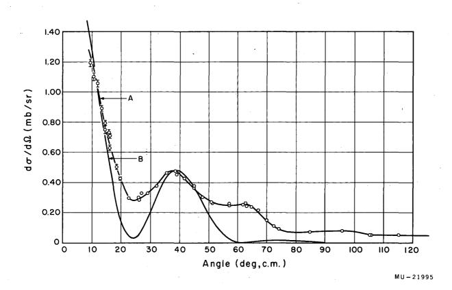
Fig. 13. Angular distribution of deuterons from formation of the ground state of Nl4. Curve A presents the experimental results; curve B, calculated results from the Glendenning equation using  $j_n$ =  $j_p$ = 1/2,  $R_O$ = 4.70 fermis.
