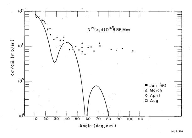
Fig. 9. Angular distribution of deuterons from formation of the 8.88-MeV level of 0<sup>16</sup>. The solid line was calculated from the Glendenning equation by using  $j_n=1/2$ ,  $j_p=5/2$ ,  $R_0=5.48$  fermis.
