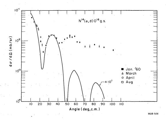
Fig. 7. Angular distribution of deuterons from formation of the ground state of 0<sup>16</sup>. The solid line was calculated from the Glendenning equation by using  $j_n = j_p = 1/2$ ,  $R_0 = 5.35$  fermis.
