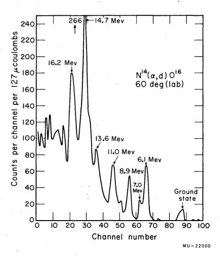
Fig. 4. Deuteron energy spectrum from the reaction  $N^{14}(\alpha,d)0^{16}$ . Q values for the various peaks are shown.
