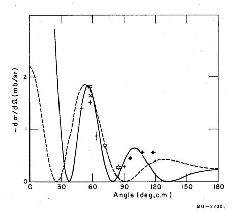
Fig. 11. Reproduction of the deuteron angular distribution from the  $\mathrm{Li}^{6}(\alpha,d)\mathrm{Be}^{8}$  g.s. transition with 11.5-Mev helium ions (Ref. 5). The solid line was calculated by using Butler theory for a stripping reaction, L = 2, R<sub>0</sub>= 9.1 fermis; the dotted line, for L= 0, R<sub>0</sub>= 5.5 fermis.
