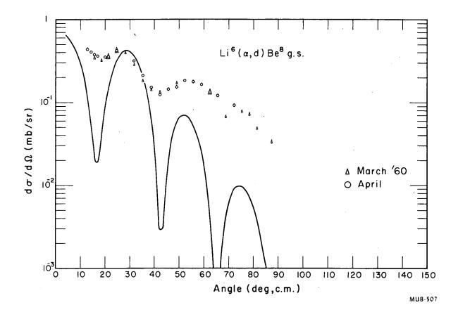
Fig. 5. Angular distribution of deuterons from formation of the ground state of Be $^{0}$ . The solid line was calculated from the Glendenning equation by using  $j_{n}=j_{p}=3/2$ ,  $R_{0}=7.6$  fermis.
