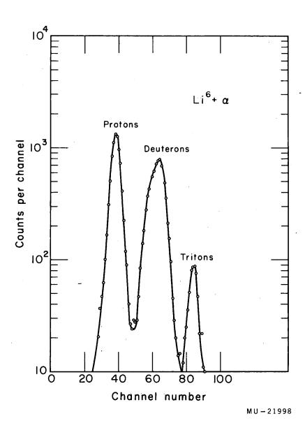
Fig. 1. Pulse multiplier spectrum from bombardment of Li<sup>6</sup> with 48-Mev helium ions.
