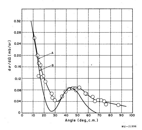
Fig. 14. Angular distribution of deuterons from formation of the 3.95-Mev level of N¹⁴. Curve A presents the experimental results; curve B, calculated results from the Glendenning equation using  $j_n$ =  $j_p$ = 1/2,  $R_0$ = 4.33 fermis.
