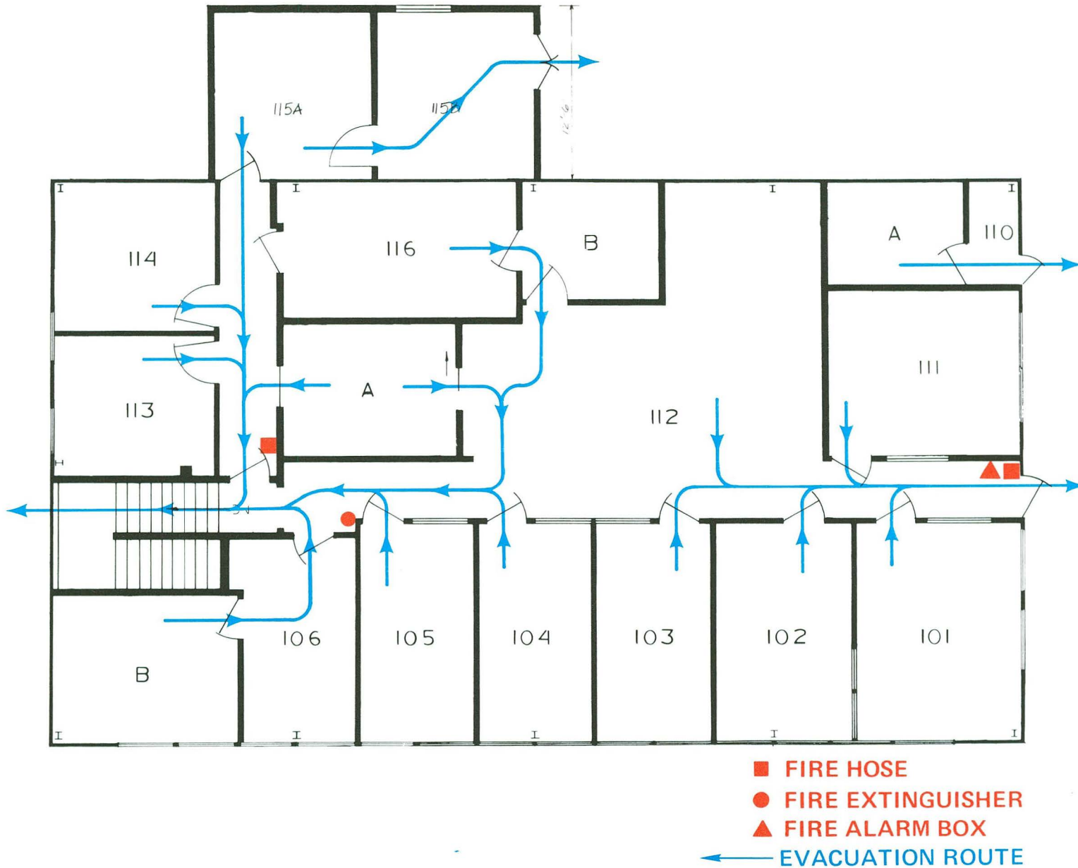
Fig. 2. Building 47, 1st FLOOR, evacuation routes and fire equipment.
