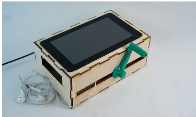
Figure 1: Our device for using Twitter requires users to constantly turn a physical hand crank to power their social media experience.
