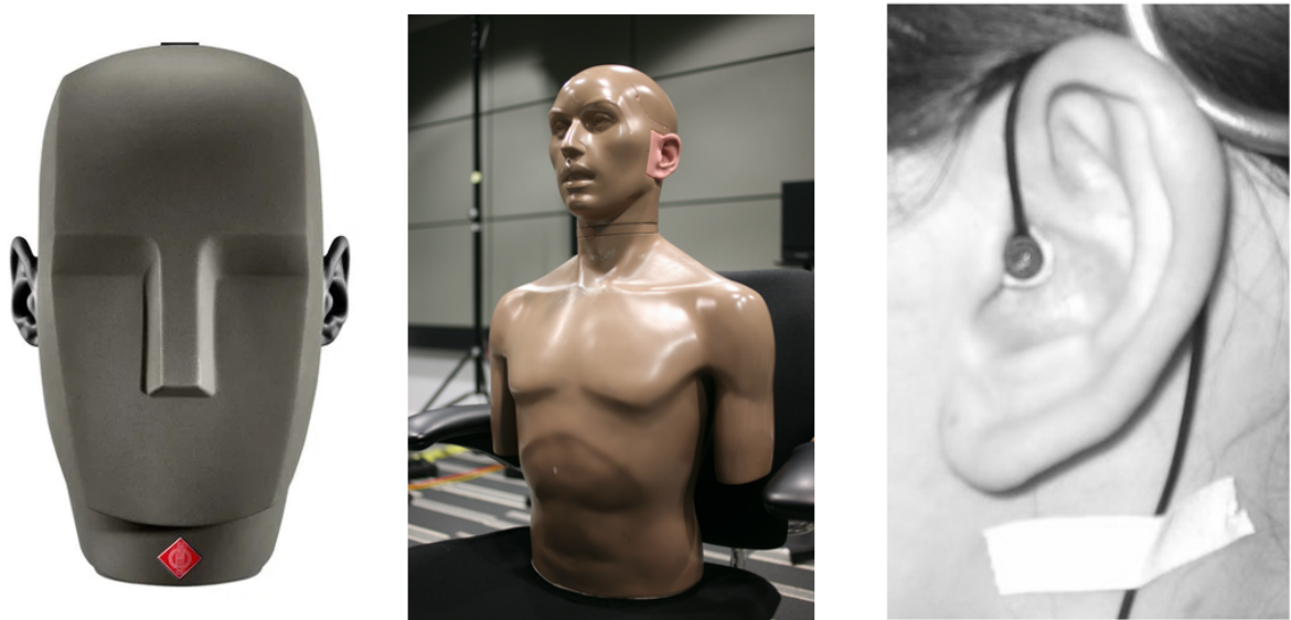
Figure 9: Left to right: Neumann KU-100, KEMAR, and in-ear binaural microphone
