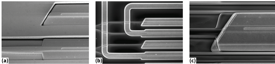
Figure 75: (a) Sample after metal deposition, before lift-off. (b) Top metal traces after lift-off. (c) Metal pad over SOA after lift-off.
