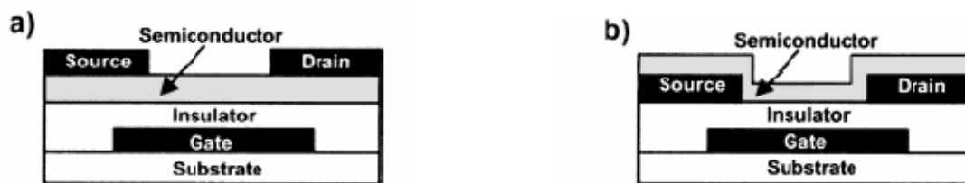
Figure 1.3. Bottom-gate OTFT device structures. (a) Top contact electrode configuration, (b) bottom contact electrode configuration.
