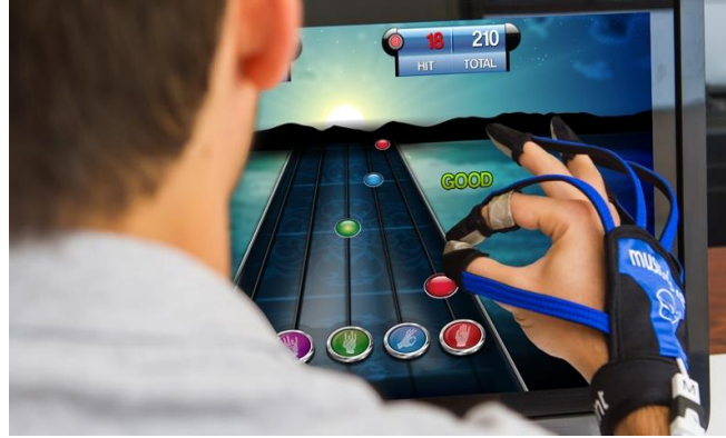
Figure 6. MusicGlove device used in study. Users viewed a musical computer game that visually cued them using scrolling notes to make specific gripping movements in time with the notes. The device detects the movements using conductive finger pads. For the present study, the game was played on a 9 in. tablet computer.
