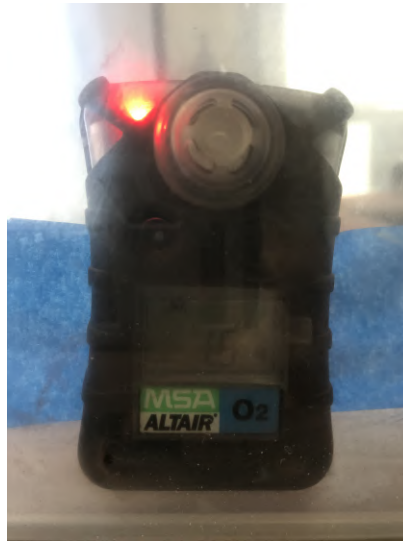
Figure 33: Oxygen sensor after Argon purge of chamber for deposition; Reading 1.5%
