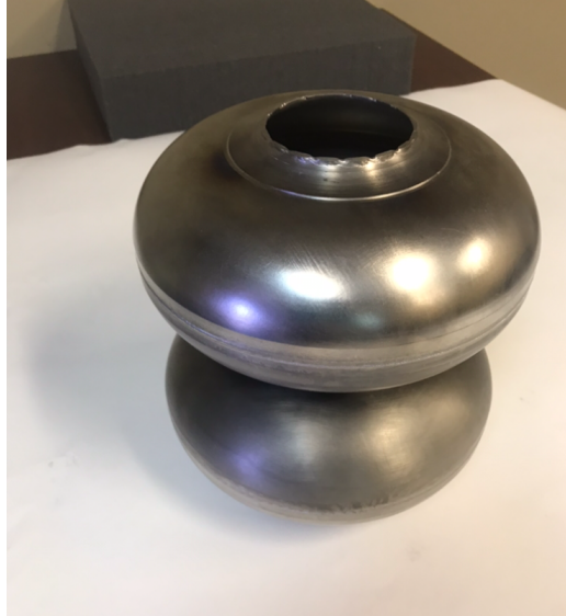
Figure 34: Approximately 8" Diameter: Nb SRF Cell used for a CAD rendering to enable Inovati to create a custom spray path
