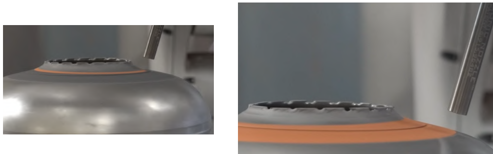
Figure 72: Spraying of complex geometry elliptical niobium SRF structure initial (Left) and final (Right)
