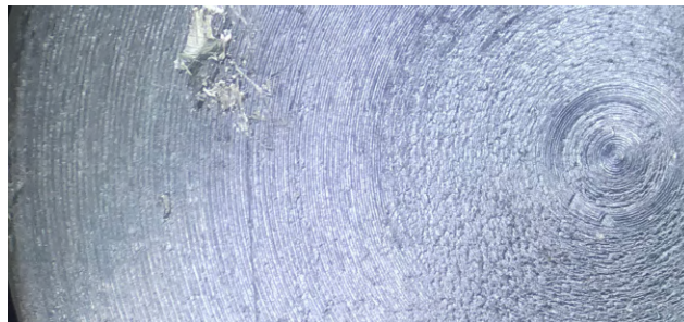
Figure 35: Image of Surface Profile of Turned Nb in Round 2 Samples - Scale is 15mm from the circular center to edge
