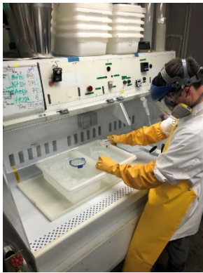
Figure 36: Left: BCP of Nb in ice bath Right: Etch rate decline with increase of Nb content
