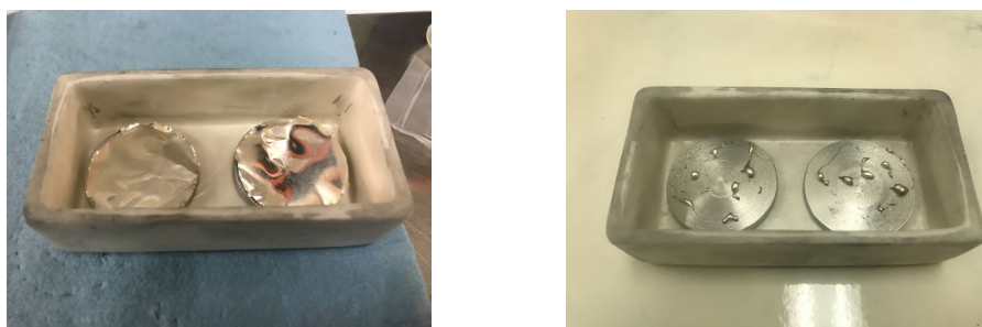
Figure 19: CuSil braze alloy Left: before braze cycle and Right: after braze cycle failed wetting of Niobium
