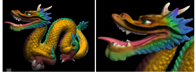
Figure 1: Our interactive 3D paint application stores paint in an octree-like structure with an effective resolution of 2048^3 (using 15 MB of GPU memory). Our system paints and renders this 817k polygon model with an octree texture at 15–20 fps and supports quadlinear filtering.
