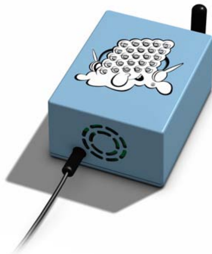
Figure 4.3. One of the air-quality sensors used in Black Cloud , an environmental alternate-reality game. Image courtesy Greg Niemeyer.
