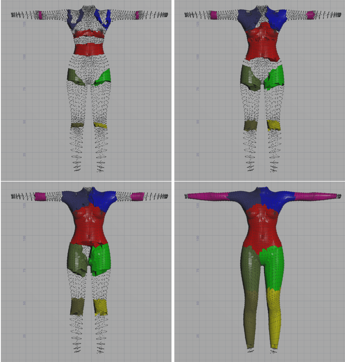
Figure 3.6: Subregion selection in the reference pose. First entire body is tetrahedralized. Each subregion is initialized as a subset of tetrahedrons that are closest to the joint of interest. The each subset is eagerly grows to their neighbors until two subregion intersect. Above figures shows initial step, step 1, step 2, and step 7.
