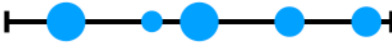
Figure 56: A diagrammatic representation of the output of the Monte Carlo. The output for for one event is a collection of dE_i (blue circles) and the space between them dx_i . The Monte Carlo is run many times, resulting in an accumulation of segments like these. Results of this type are referred to as the “base 1D” Monte Carlo.
