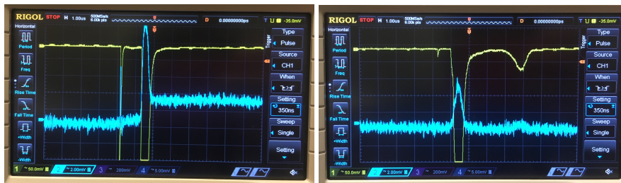
Figure 149: Examples of the charge amplifier mirror effect on one anode segment. The example (left) is an event where charge is collected on the anode segment, and so the charge amplifier signal trace shows a step. The example (right) shows the charge trace mirroring the PMT , but with no charge collected on the anode segment.
