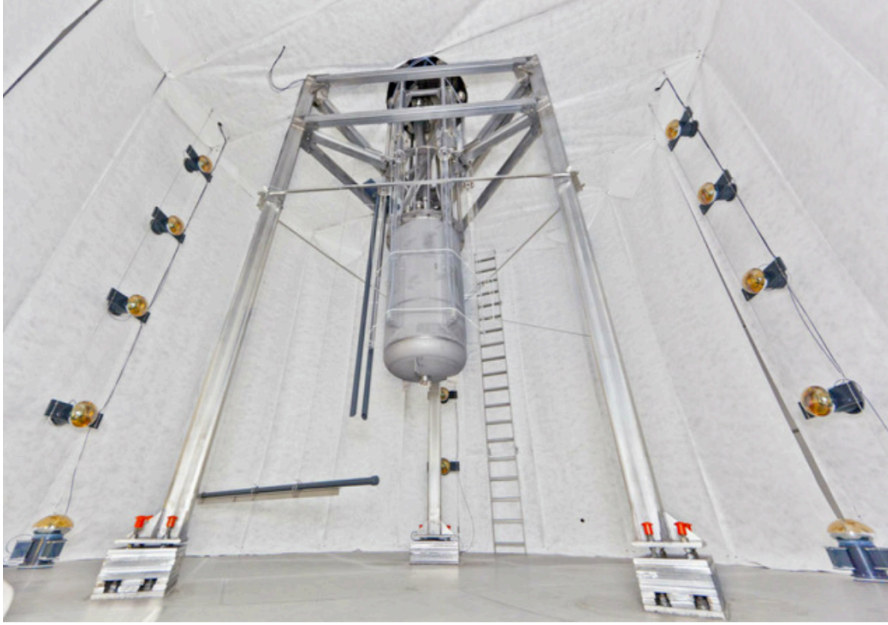
Figure 33: A photo of the LUX detector installed inside the water tank. Photo credit Mark Kapust.
