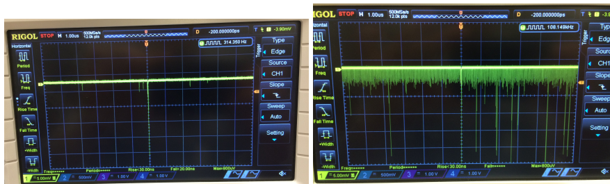
Figure 112: Oscilloscope showing baseline rate of single photons (left) compared to a high rate of single photons (right) caused by the high voltage feedthrough. In both figures, the vertical scale is 5.00 mV/div and the time scale is 1.00 \mu s/div.
