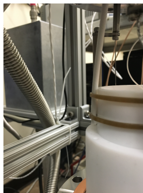
Figure 115: Effect of holding the feedthrough in place with PEEK zip ties was explored. The voltage properties were not found to improve, but neither did they degrade.
