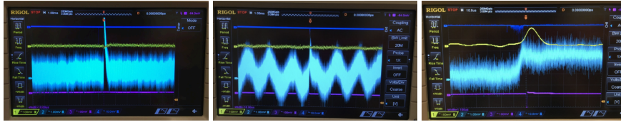
Figure 101: left) Event showing charge amp with detector -100 C, 1.5 bar, gas only (time scale 1.00 ms/div). (middle) Effect of circulation pump on charge amp is to cause 500 Hz oscillation noise (-100 C, 1.5 bar, gas only (time scale 1.00 ms/div)). (right) Same event as (middle), but zoomed-in time scale (10.0 \mu s/div). In all figures, cyan is the raw charge signal (1 mV/div), yellow is the shaped charge (100 mV/div), blue is the PMT (10 mV/div) and magenta is the NIM trigger (100 mV/div).
