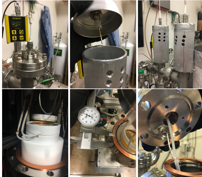
Figure 120: Top: (left) Sealed top connection with liberal epoxy use. A male Bendix pin was soldered to the cable conductor. (middle) SHV connector with female Bendix to mate with feedthrough (right) Grounded safety housing with SHV connector. Bottom: (left) Ends of the feedthrough were held in the Teflon stack. (middle) Close up showing cable conductor, PTFE dielectric, and grounding sheath pulled back. The calipers are measuring the length of exposed conductor. (right) Grounding scheme for feedthrough cables at the top of the CF tower.
