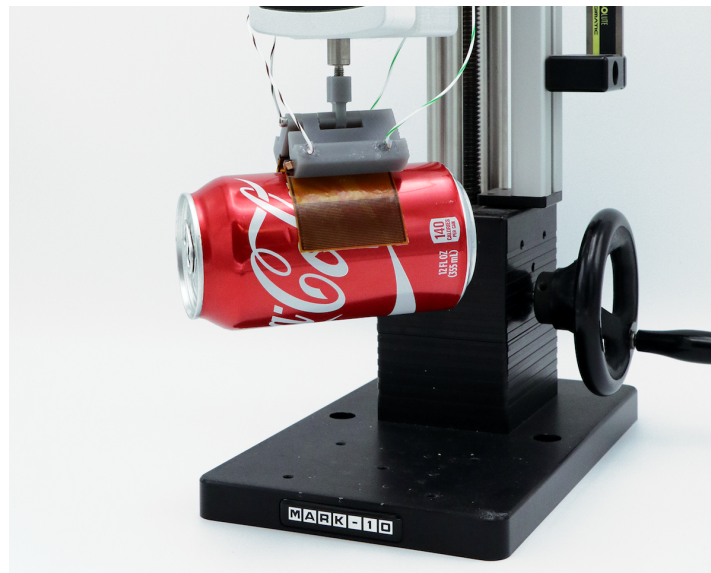
Figure 5.11: Prototype gripper with two rectangular hybrid adhesive fingers, grasping and lifting a full soda can (3.6 N).
