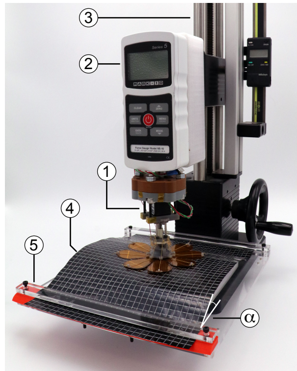
Figure 5.7: Gripper force characterization set-up. The electrostatic gripper (i) is mounted to the force gauge (ii), which slides along the z-axis stage (iii). The film (iv) being tested is secured in a bracket assembly (v) below the gripper.
