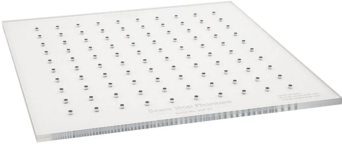
Figure 5.7: Beam stop array consisting of a regular array of small lead discs embedded in a low-attenuation supporting plate.
