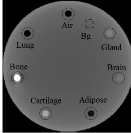
Figure 4.16: Contrast rod slice comparing HU values and CNR of inserts composed of lung, bone, cartilage, adipose, glandular, and brain tissue across the sampling densities tested.
