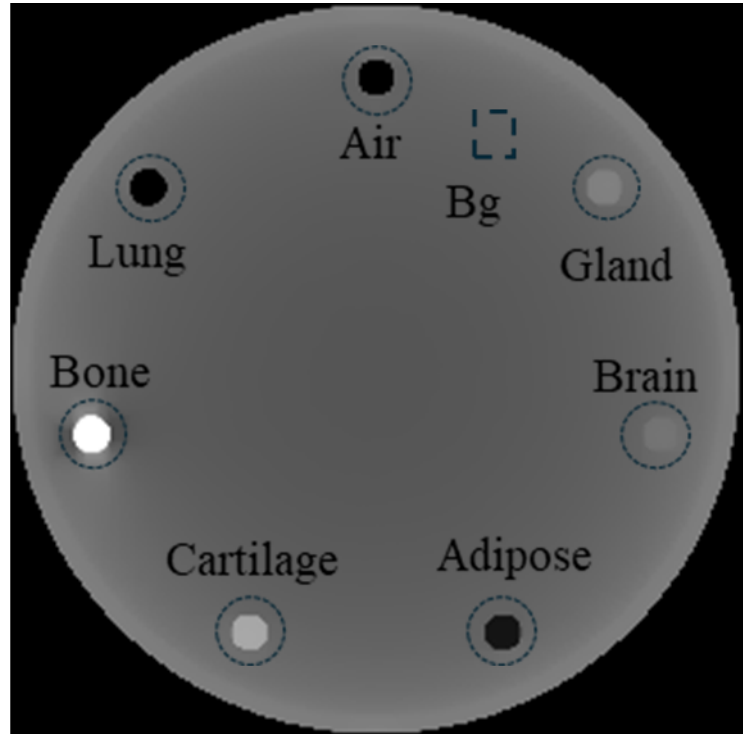
Figure 4.11: Contrast comparison slice with material insert ROIs and water-equivalent background ROI used for CNR and HU accuracy calculations.
