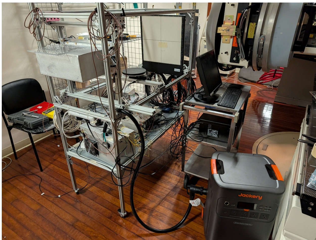
Figure 5.2: Latest iteration of the benchtop CBCT system showing the redesigned benchtop cage, portable high power supply, new X-ray source-controller, interfacing computer, inherited detector, and new rotary stage.
