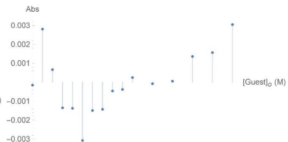
Figure 6.86. Fitting curves and plots of residual magnitude obtained when fitting the UV binding data for C 6 -SH with cage 2.1 to the 1:1 binding model.
