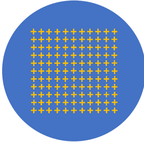
Figure A-9. Mark matrix layout after release 1st handler. The blue background is PDMS and yellow crosses are gold marks.
