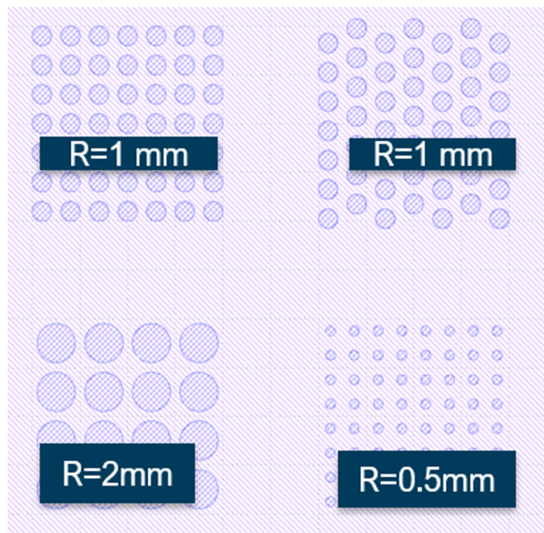
Figure 2-6 Experimental design comparing different electrode radii and stacking configurations.
