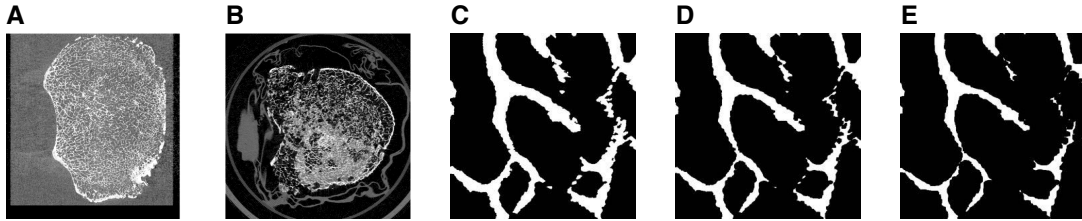
Figure 4.2: Example raw micro-CT image slices and comparison of thresholded and eroded images. A: Example 9 \mu\text{m} -resolution micro-CT image slice from vertebral body dataset F60L3. The image slice lies in the transverse plane and is 56.1 mm wide and 59.4 mm long. B: Example transverse slice from osteoporotic vertebral dataset AE15TH11, 52.0 mm \times 52.0 mm. Image contrast has been increased in panels AB to improve visibility. CDE: 5 mm \times 5 mm section of micro-CT image, eroded at various stages to simulate effect of osteoporosis. C: Baseline thresholded (healthy) section. D: The same section as in C, eroded with radius of 2 voxels (osteopenic). E: The same section as in C, eroded with radius of 4 voxels (osteoporotic).
