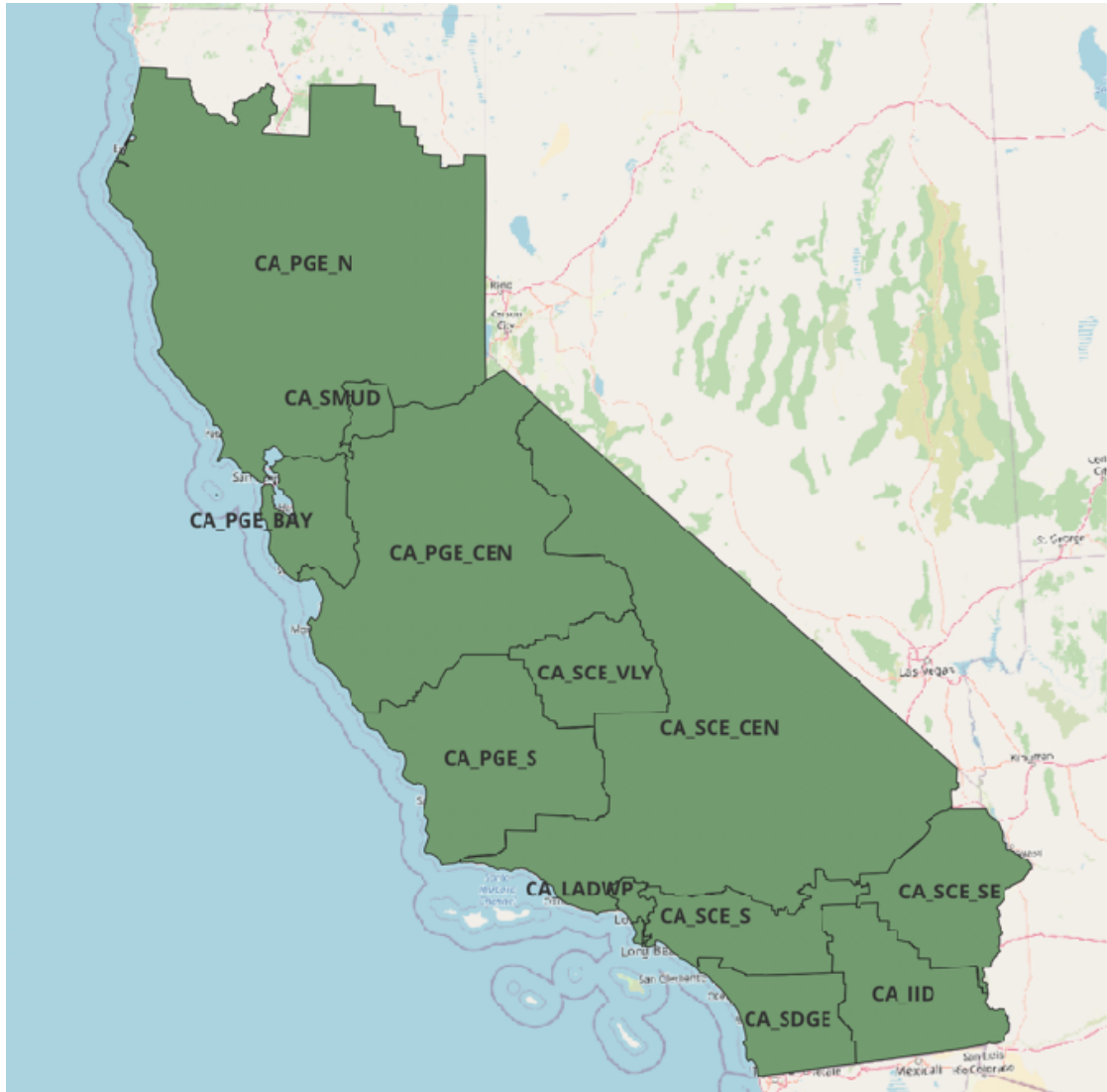
Figure 4.1: Grid topology proposed for California. The shape and area of the load zones are similar to those previously developed by the Switch-WECC team.
