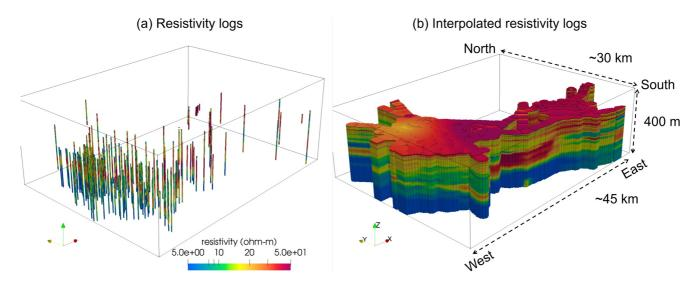
**Figure 4.** Interpolation of resistivity logs. (a) Vertically upscaled resistivity logs at 152 well locations. (b) 3D interpolated volume of the resistivity displaying result of the interpolation. The vertically upscaled resistivity logs were interpolated to the discretized layers at all sounding locations resulting in  $\rho_{int}^{log}$ . For a visualization purpose, we interpolated the  $\rho_{int}^{log}$  to the 3D grid as shown in Figure 6b.
