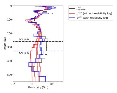
**Figure A6.** Six layered-resistivity models recovered from 1D AEM inversions with different prior models. Red and blue lines distinguish whether the upscaled resistivity log was used as a reference model or not. Black line shows the upscaled resistivity log. Black and blue dashed lines show the DOIs with threshold values of 0.4 and 0.9, respectively.
