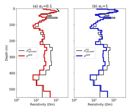
**Figure A5.** Recovered layered-resistivity models from inversions by using the upscaled resistivity log as a reference model with variable  $\alpha_s$  values: (a) 0.1 and (b) 1. Black line shows the upscaled resistivity log. Both the smoothness constraint and reference model were used for the regularization function.
