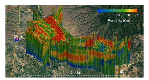
**Figure 5.** Three-dimensional display of subsurface variation in electrical resistivity in Butte and Glenn Counties in the Central Valley of California, USA., obtained through the processing and inversion of AEM data. The inverted 1D resistivity models imaging the top  $\sim$ 400 m of the subsurface in the study area are displayed at AEM sounding locations. This resistivity model corresponds to Inversion 6 in Table 2.
