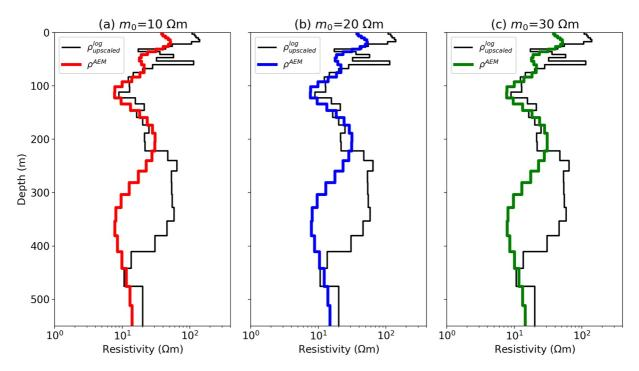
**Figure A2.** Recovered layered-resistivity models from inversions with variable initial models: (a)  $10 \Omega m$ , (b)  $20 \Omega m$ , and (c)  $30 \Omega m$ . Only the smoothness constraint is used for the regularization function.
