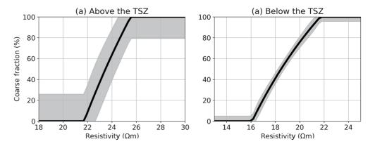
**Figure 12.** The relationship between resistivity and coarse fraction: (a) above and (b) below the top of the saturated zone (TSZ). Gray shaded region indicates the standard deviation of the coarse fraction illustrating the uncertainty of the transform when converting resistivity values to coarse fraction.
