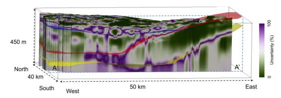
**Figure 11.** The estimated uncertainty in sediment type from AEM data in a 3D view. The 3D uncertainty extends from the vertical section A–A′ the location of which is shown in Figure 2, and extends to the north. Blue dashed lines indicate the location the A–A′ vertical section in the 3D view.
