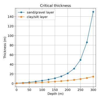
**Figure 7.** The critical thickness of a layer as a function of depth. The critical thickness is the required thickness of a layer, embedded in a homogenous background, in order for the layer to be detected by AEM data. Blue curve: a sand/gravel layer in clay/silt background. Orange curve: a clay/silt layer in a sand/gravel background. The resistivity values used for clay/silt and sand/gravel were 16 and  $22 \ \Omega m$ , respectively.
