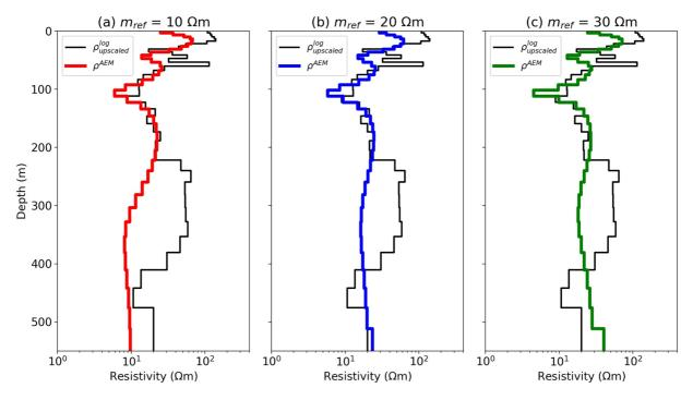
**Figure A3.** Recovered layered-resistivity models from inversions with homogeneous reference models: (a)  $10 \Omega m$ , (b)  $20 \Omega m$ , and (c)  $30 \Omega m$ . Both the smoothness constraint and reference model were used for the regularization function.
