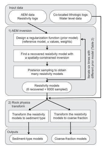
**Figure 3.** Flow chart for the estimating ensemble of sediment-type and coarse-fraction models from AEM data and other ancillary data sets including resistivity logs, co-located lithologic logs, and water level data.
