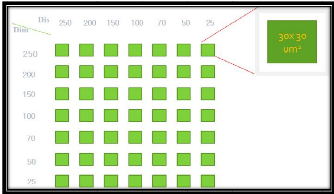
Figure 3.3.1: Schematic of design structure used to determine proper dosage trend. Distance varies from 250 nm to 25 nm, while pattern dimensions change from 250 nm to 25nm at a same time. The entire pattern exposed covers an area of 30x30 \mu\text{m}^2 and is surrounded by areal reference mark.
