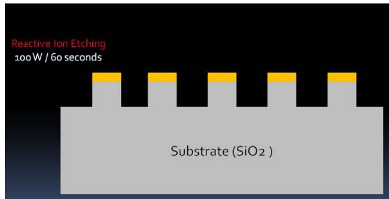
Figure 5.3.6: Main milling processing with RIE. Silicon dioxide substrate is milled under 100 Watt power for 60 seconds, with \text{CHF}_3 of 50 sccm. The depth of milling is around 100 nm confirmed by AFM analysis.
