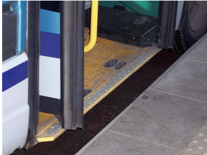
Figure 2. TEOR Precision Docking at Bus Stop
