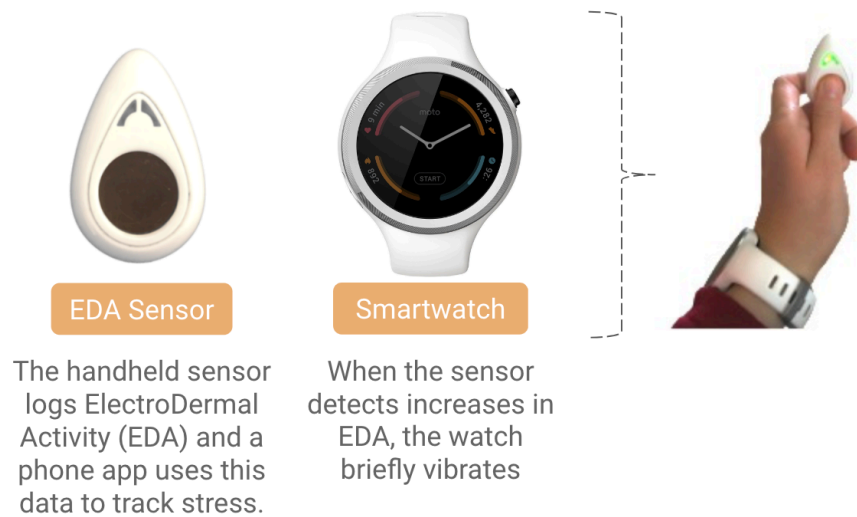
Figure 3. The pip is held between the thumb and forefinger and a smartwatch is worn on the left wrist. When the pip detects an increase in ElectroDermal Activity (EDA), the smartwatch briefly vibrates.
