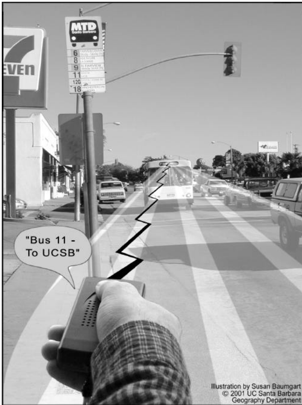
Figure 2.7 Using RIAS to Identify an Approaching Bus
