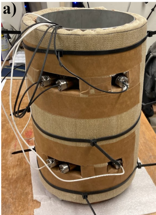
Figure 2.26: a) A photo of the inner layer thermal insulation blanket with a thickness of 2 cm. b) Thermal conductivity of the insulation material – Aspen Aerogels Cryogel x201. Figure modified from the product’s data sheets.
