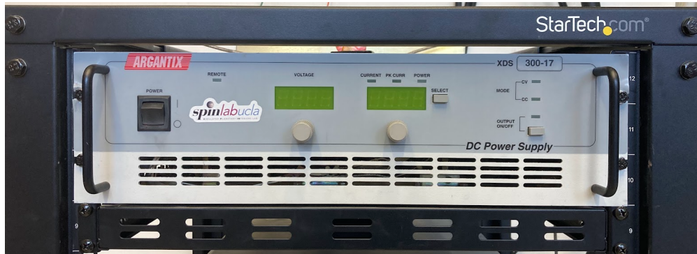
Figure 2.5: Argantix XDS 300-17 power supply for providing heating power up to \sim 5 kW into the system. The Magna-Power power supply for the magnet is located directly below this power supply in the same rack.
