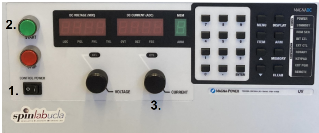
Figure 2.24: Magna Power Supply control panel. The numbers indicate the proper steps for manual current controls.
