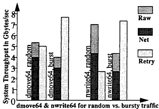
Figure 6: Comparison of switch throughput for random and bursty traffic, 8_R \times 8_R multi-stage network.
