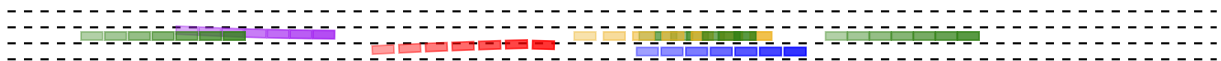
(c) The ego vehicle fails to do a lane change maneuver. A fast vehicle (yellow one) drives “through” a slow vehicle (one of the green ones). The change of vehicle ft in the controller makes the barrier function h_{ft}(\mathbf{x}, t) 's value change suddenly. This scenario will not happen in real world.
