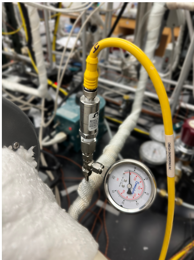
Figure 6.7: Pressure sensor lines are located vertically and not heated to prevent damage to the pressure transducers. Placing material in the tube to prevent condensed water from falling in to the hot tube below, eliminated potential spikes caused by condensation in these line.
