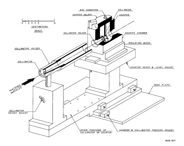
Fig. 2. Counter and gas target collimation.
