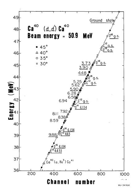
Fig. 7. Energy scale for energy spectra from  $\theta_{\text{lab}} = 30^{\circ}$  to  $\theta_{\text{lab}} = 45^{\circ}$ . Only  $\theta_{\text{lab}} = 30^{\circ}$ , 35°, 40°, and 45° are plotted. The ordinate is the calculated energy assuming incident beam energy of 50.9 MeV, and the Q values given in Table I. The abscissa is the channel of the peak. The states underlined were used to determine the line.
