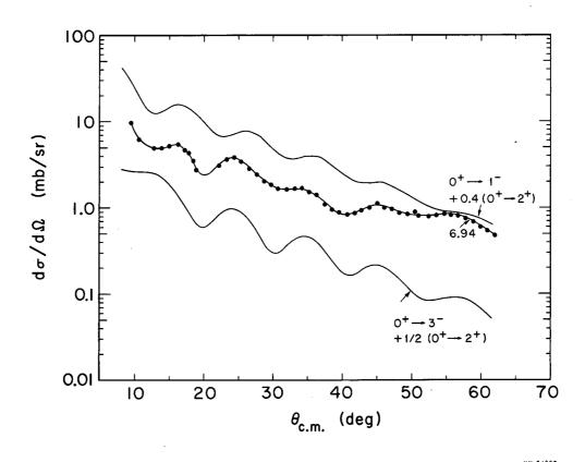
Fig. 13. The Ca<sup>40</sup> 6.94-MeV state experimental differential cross section compared with two Austern and Blair angular distributions for a doublet. The upper curve is a sum of  $(0+\to 1-)$  and  $(0+\to 2+)$  in the ratio of 5 to 2. The lower curve is a sum of  $(0+\to 3-)$  and  $(0+\to 2+)$  in the ratio of 2 to 1. Except for a few small angle points the lower curve is more in phase with the experimental curve.
