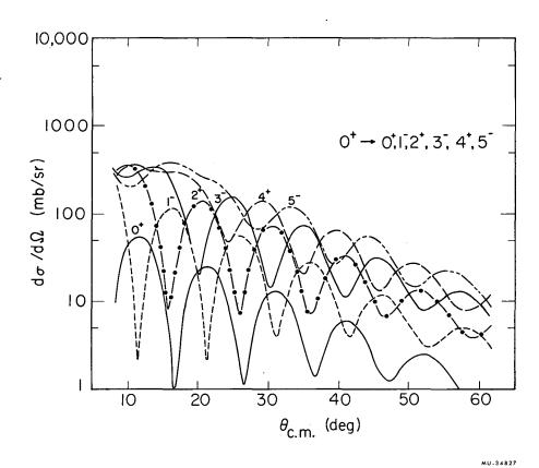
Fig. 19. Austern and Blair model angular distributions calculated with parameters determined from the Ca $^{140}$  elastic differential cross section in Fig. 3. Transitions  $0+\to 0+$  through 5- are plotted with the first maximum of the regular oscillations indicated on each curve. From a spectroscopic standpoint this differentiates the different angular momentum transfers.
