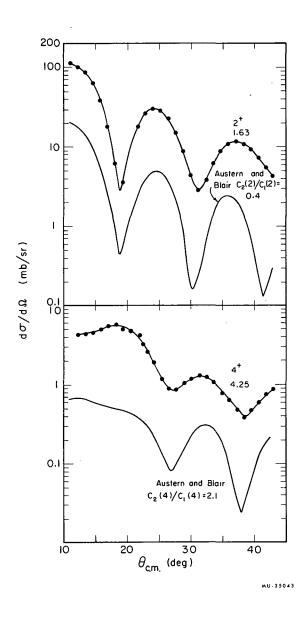
Fig. 14. Ground state band 2+ and 4+ experimental and theoretical angular distributions in  ${\rm Ne}^{20}$ .
