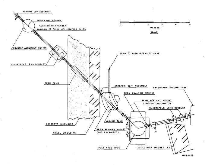
Fig. 1. Beam optics system of 88-in. cyclotron, cave 1.
