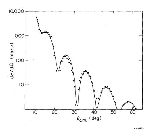
Fig. 17. Parametrized phase shift fit to Ca elastic differential cross section with the parameters; L = 16.7;  $\Delta$  = 1.15; A = 0.66; B = 1.51; D = -1.92. The parameters are described in the text.
