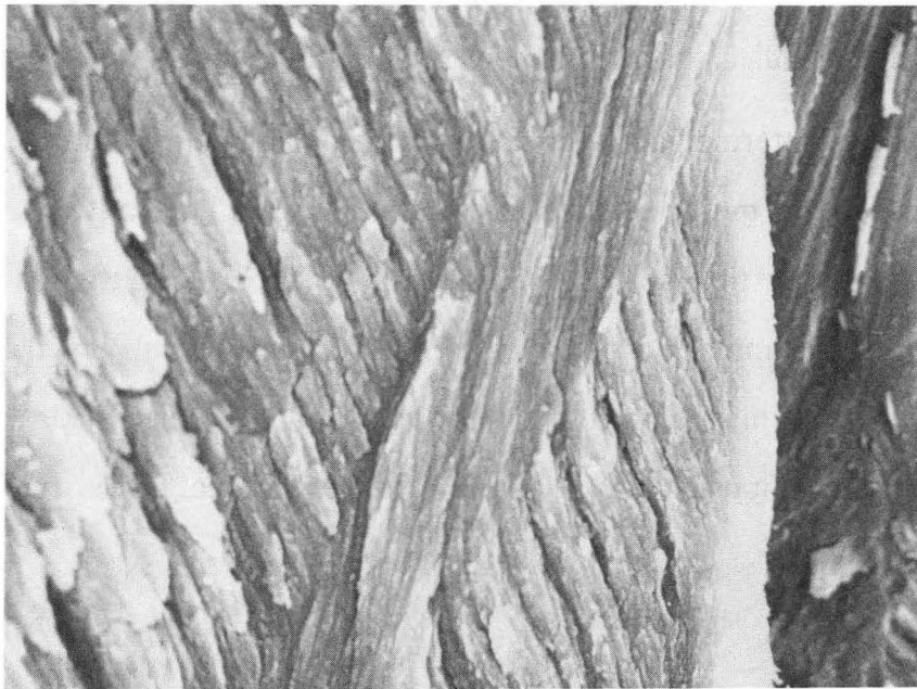
Fig. 2--a higher magnification view of the outer layer in Fig. 1. The ridges and cracks are portions of rod bundles and cylindrical pores.
