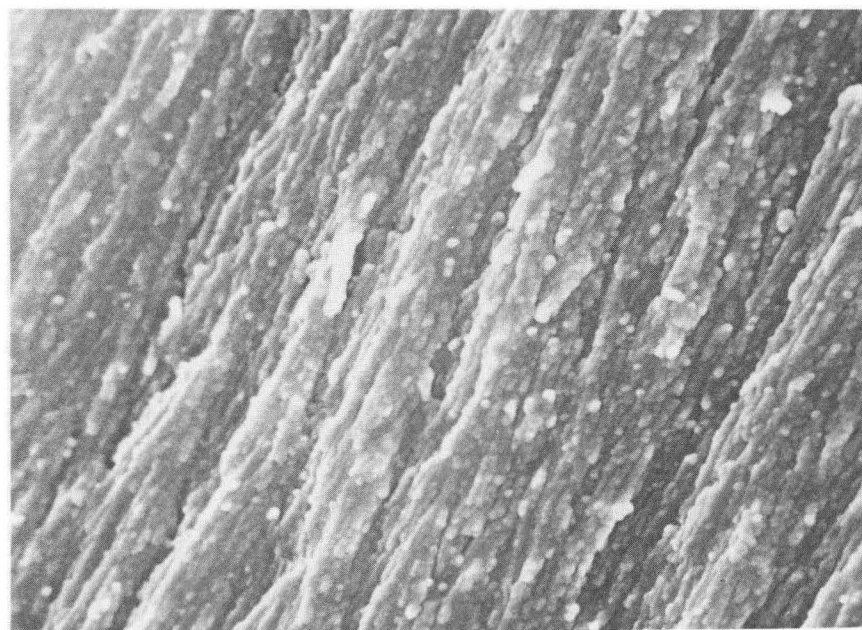
Fig. 6 --a high magnification view of the type of outer layer surface shown in Fig. 5. The ridges and valleys are portions of rod bundles and cylindrical pores.
