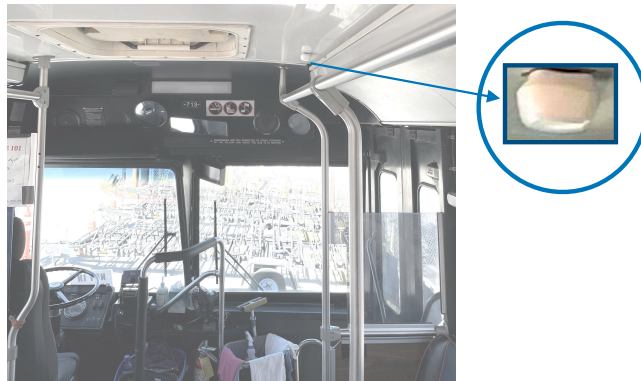
Figure 2: Example of placement of a BLE beacon (Kontakt Tough TB15-1) on the ceiling of the shuttle bus.
