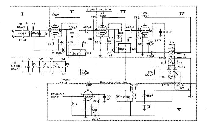
Fig. 29. Schematic diagram of the null detector showing divisions between the amplifier stages in the constructed unit.
