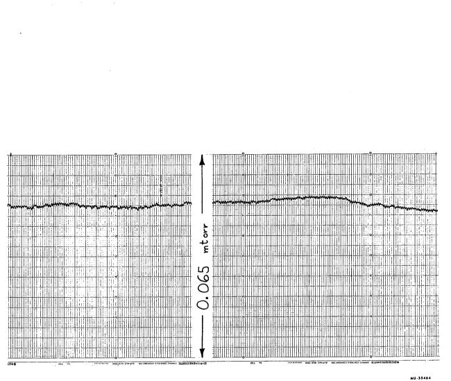
Fig. 41. Typical short term and long term stability curve for Decker-Lamers-Rony No. 1 system. Signal attenuation factor = 1.0 and recorder output potentiometer setting = 2.00 turns (total time = one hour).
