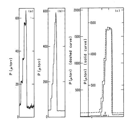
Fig. 42. Typical recorder-chart calibration data: (a) DLR No. 1, attenuation factor = 1.0, and recorder output setting = 2.00 turns; (b) DLR No. 1, attenuation factor = 0.1, and recorder output setting = 3.00 turns; (c) DLR No. 1 (solid curve) and DLR No. 2 (dashed curve), identical attenuation factors = 0.02, and identical recorder output settings = 3.00 turns.
