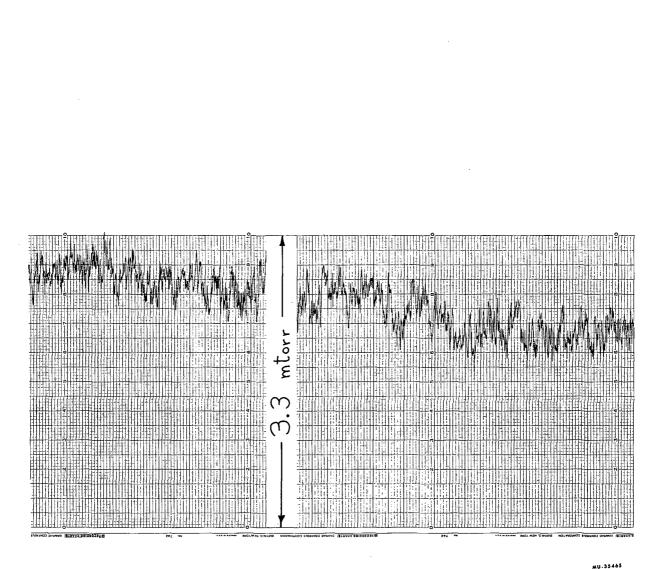
Fig. 40. Typical short term and long term stability curve for Decker 306-2A sensor and 306-2 meter (total time = one hour).
