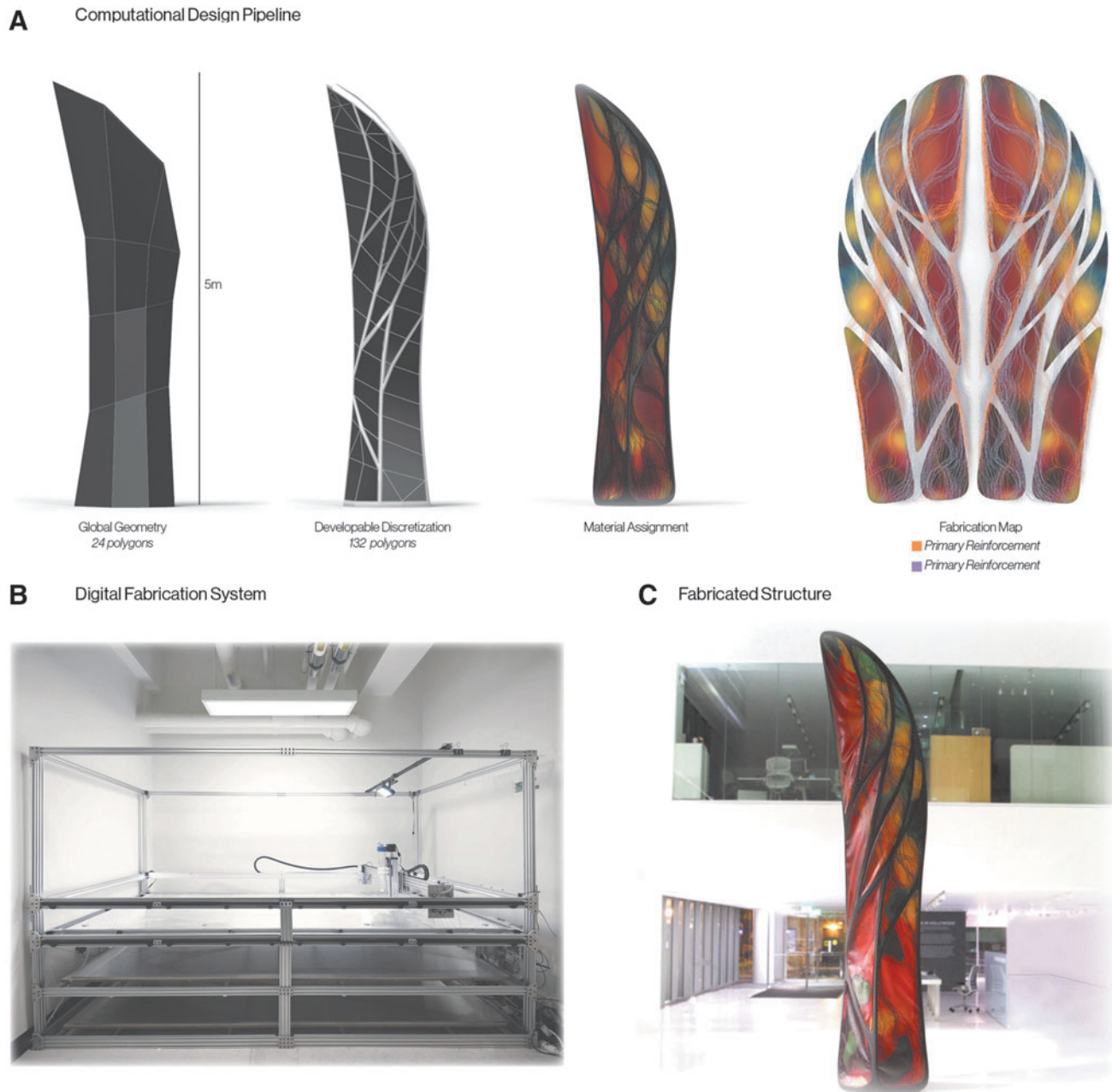
FIG. 5. Fabrication of a large-scale prototypical membrane structure with both continuously graded and discrete embedded material transitions demonstrates efficacy of the described methods across scales of fabrication. A 5-m-tall base-geometry was processed into developable panels and assigned colored gradients of materials, as well as embedded reinforcement patterns, with the largest panel spanning 2 m ( A ). The panelized structure was fabricated by affixing the described extrusion system to a 2 m by 4 m CNC gantry ( B ) and supported by a rigid acrylonitrile butadiene styrene (ABS) scaffold ( C ). Base layers containing 32% pectin, 0% to 6% chitosan, and 1% acetic form a flexible skin with gradients of color and strength. A secondary network, embedded as a reinforcement pattern within the base layer, consists of 32% pectin, 8% chitosan, 15% cellulose, and 1% acetic acid and provides additional reinforcement to the structure. CNC, computer numerical control.
