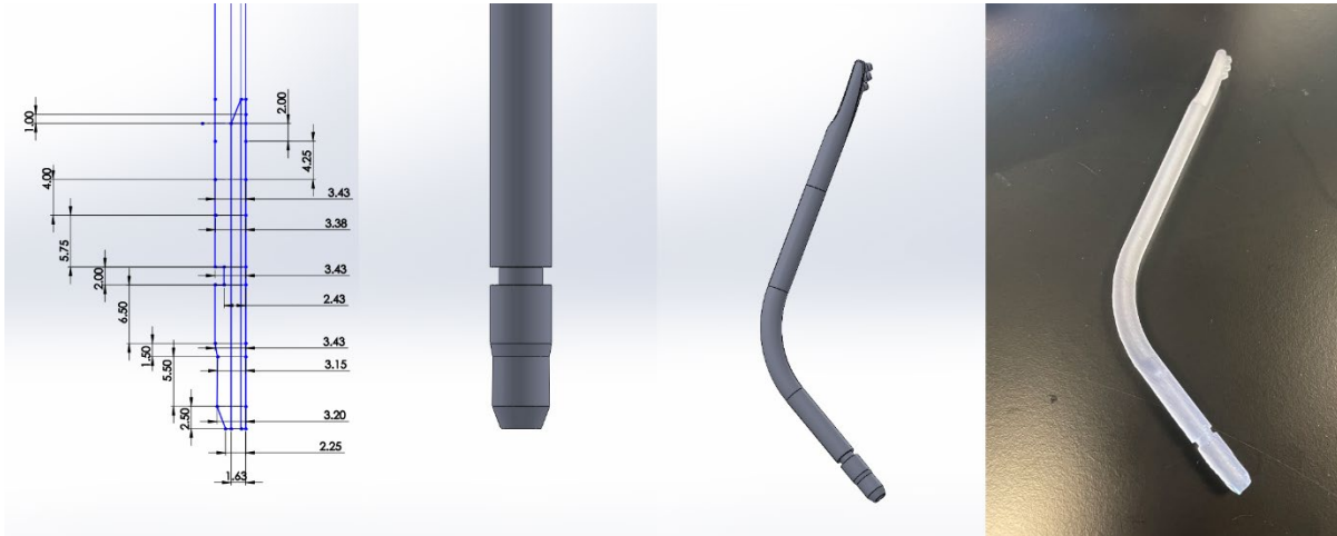
Figure 2.2 Design stages of a custom shower head.
