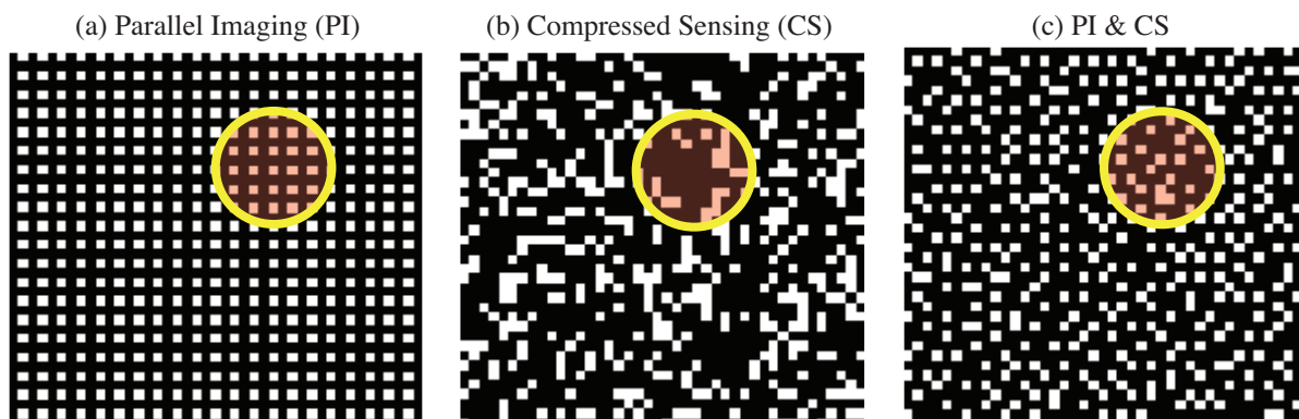
Figure 6.6: (a) Uniform undersampling (Not incoherent) harms compressed sensing reconstruction. (b) Random undersampling (bunched or too many “holes”) harms parallel imaging reconstruction. (c) Locally uniform and globally random undersampling (Poisson-Disc Sampling).
